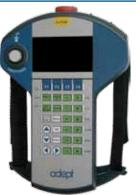
The Adept T20 manual control pendant provides an ergonomic and durable package with which users can manually teach the robot system. All gripping and holding positions enable comfortable and fatigue-free operation. Select features include
